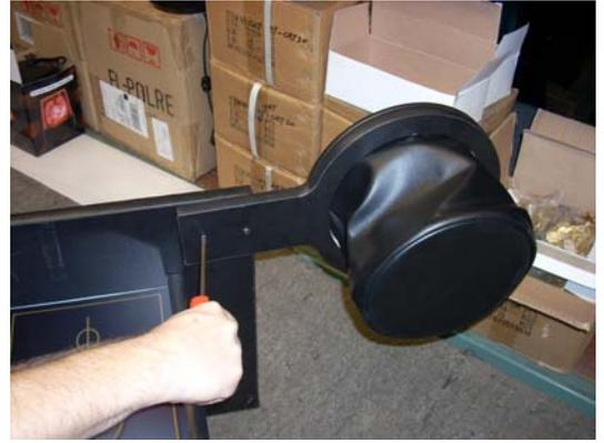
**Step 2: Stand the base upright and set the machine on the base. Tip the machine forward and insert the machine power cord through the hole in the top of the base. Then set the machine back down flat on the base.**
