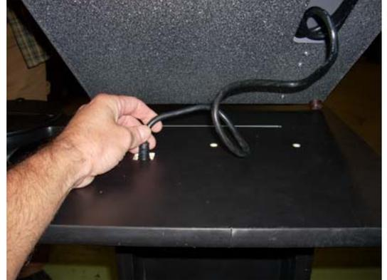
**Step 3: Plug the machine power cord into the outlet located on the rear of the stand. Plug the main power cord at the bottom of the stand into a wall outlet and turn the power switch on.**
