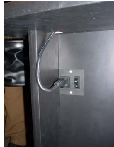
**Step 4: Attach the rotating beacon to the lid of the machine and plug it in to the outlet on the rear bottom of the machine.**
