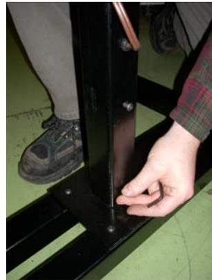
Attach the handle to the rear of the main pole with (2) 10-32 X 1/2" (L) screws about 12 inches below the top of the pole on the rear side.
