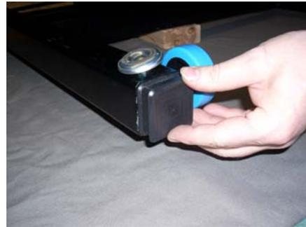
Flip the base over on to its levelers and install the pole support to the center of the base using (4) 1/4-20 X 1/2" (M) screws. **Note that the single 1/2" hole in the support must face forward away from the wheels.** Tighten the screws securely.
