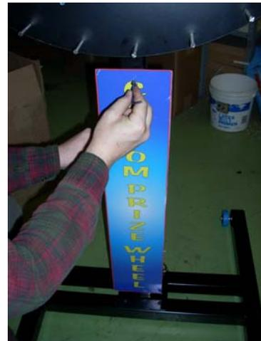
Install the wheel art plackard to the wheel. Make sure to line the six mounting holes on the plackard with the six screw inserts in the wheel before sliding the plackard over the pins. Secure the plackard to the wheel with (6) 10-32 X 1/2" (L) screws.
