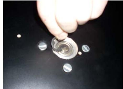
Install the (24) clicker pins (E) to the wheel. Insert the pins through the front of the wheel and secure with a capnut on rear side. Do not over tighten.
