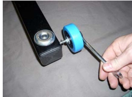
Install a tube cap (A) at each corner. You may have to apply a little silicone to each cap for a more permanent installation.
