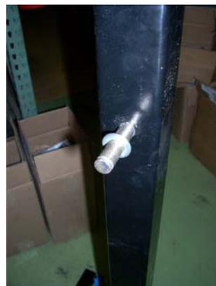
Install the wheel to the wheel pin by sliding the bearing hub over the pin and pushing the wheel on to the pin as far as it will go. **The bearing hub should be at the rear of the wheel.**
