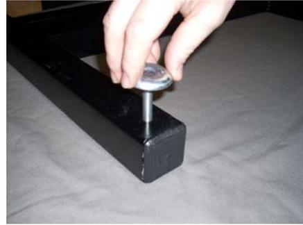
Slide a lock washer (D) over the bolt of each wheel assembly (C) and tighten the wheel bolts securely to the base. This will be the **rear** of the base.
