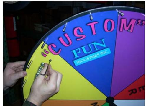
Install the header plackard to the header with (2) 10-32 X 1/2" (L) screws.
