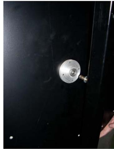
Secure the wheel to the pin by installing the C-clip (G) to the front side of the pin. The clip will snap into the slot cut in the pin. You may need to push the clip into place with a screwdriver.
