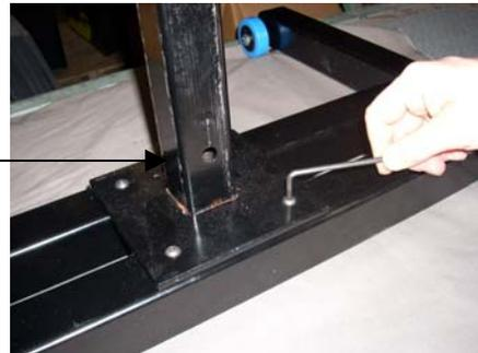
Slide the main pole on to the support with the power cord at the bottom and towards the rear.
