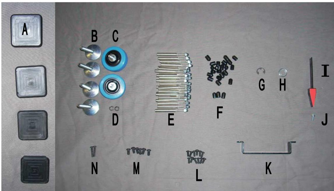
Set the main base unit on a table. Install the 4 leg levelers (B) into the tapped holes at each corner of the base. This will be the **bottom** of the base.
