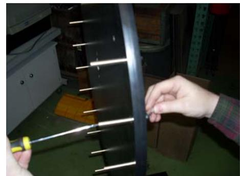
Install the header to the front of the main pole above the wheel with (2) 10-32 X 1" (N) screws.
