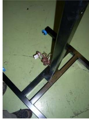
Attach the main pole to the support with (2) 1/4-20 X 1/2" (M) screws below the power cord at the rear of the pole and tighten securely.
