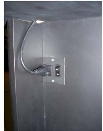
Plug the 3-way cord adapter into the outlet on the lid of the machine then plug the beacon and overhead light into the 3-way adapter.
