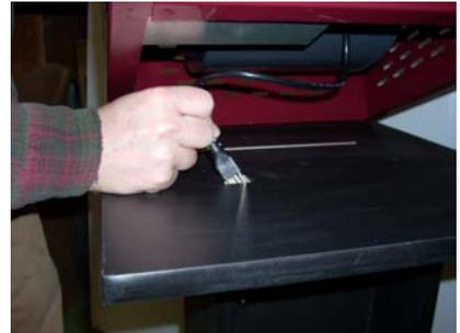
Plug the machine power cord into the outlet in the rear of the base unit. Notice the main power switch is located here. Then plug the main power cord at the bottom of the base into a wall outlet and turn the power switch on.
