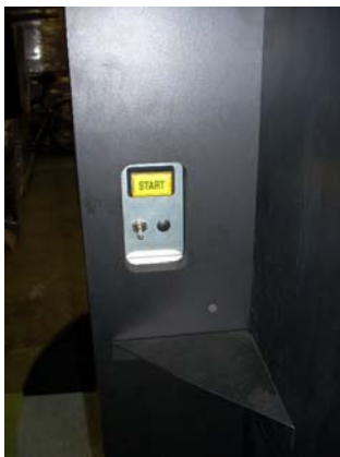
1. Operator Pushes Start
